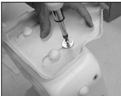
4. Using a sheet metal screw and washer, attach the Bo Villa securely to the Hanging Block. (This is a cut out of a Bo Villa)
